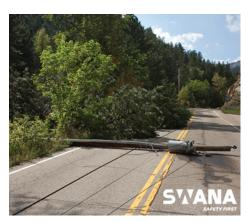
The safest plan is to never go near a downed or fallen electric power line, and to treat all electrical wires as unsafe until proven otherwise. <u>Learn more on OSHA's website.</u>
